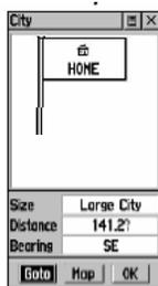
6 - Use the THUMB STICK button to select GOTO at the bottom of the screen.
