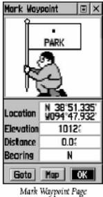
2 – Your waypoint is automatically assigned a three-digit number. To change the name of the waypoint, use the THUMB STICK button to highlight its name. Use the THUMB STICK to select the new name for the waypoint.
