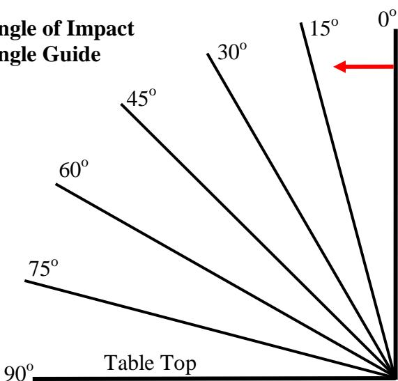
Tape this card to the side of a table so that the table top is level with the  $90^\circ$  line.
